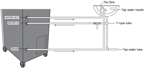
5. Once the pipe connection is finished, open the valve of water supply line so that water is supplied. At this time, as water is discharged only when the air—conditioner is operated, check whether water is discharged from the drain hole.
